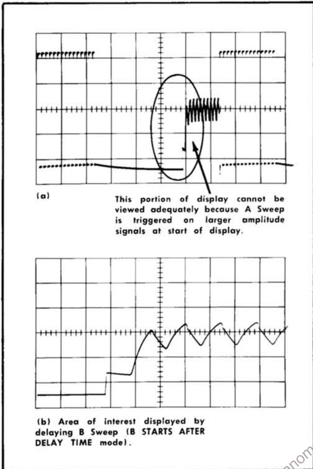
Fig. 2-21. Displaying a complex signal using delayed sweep.
