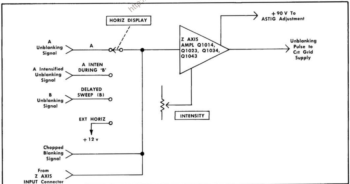
Fig. 3-11. Block diagram of Z Axis Amplifier circuit.
