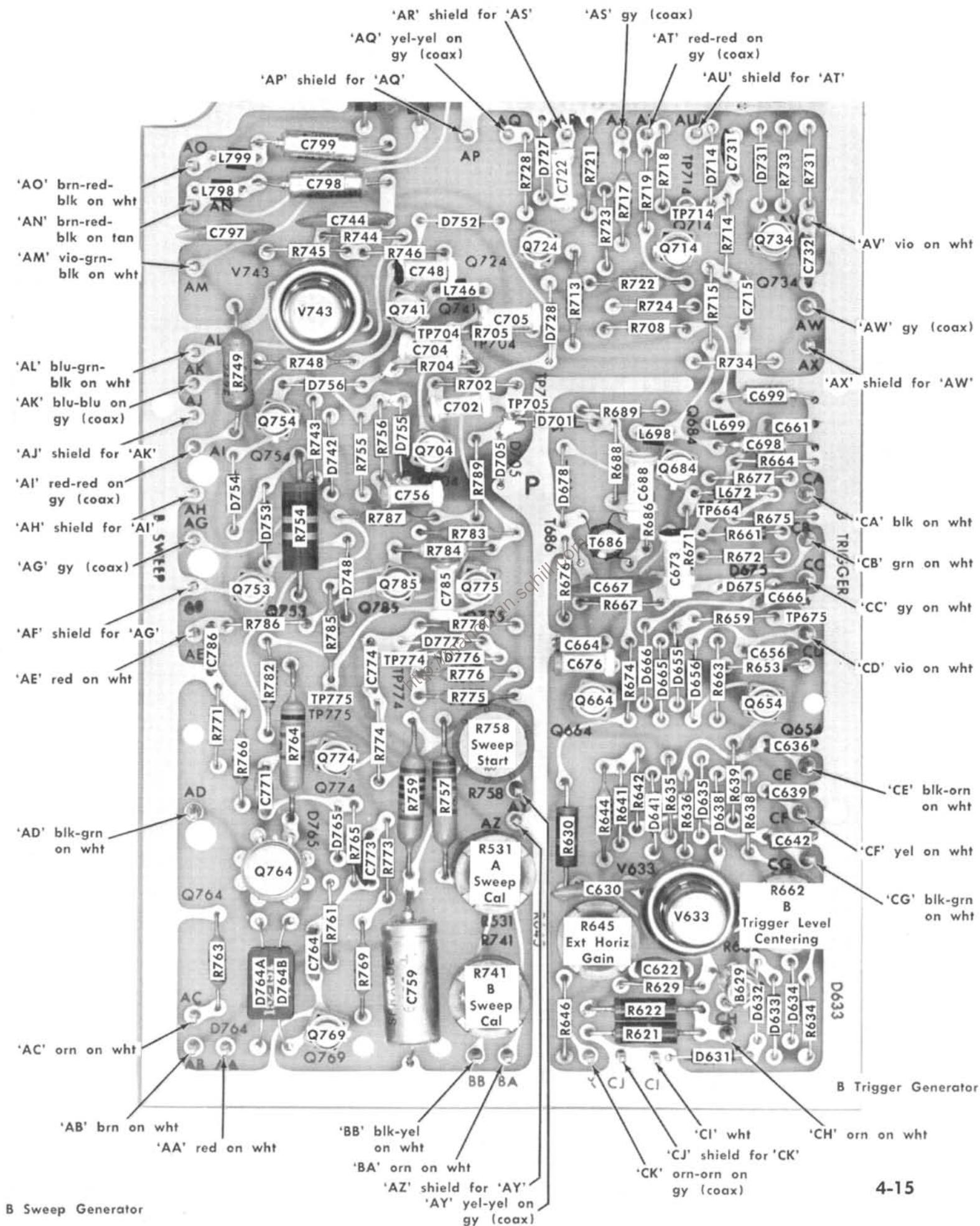
Fig. 4-10. B Trigger Generator and B Sweep Generator etched-wiring board (partial B Sweep board).
