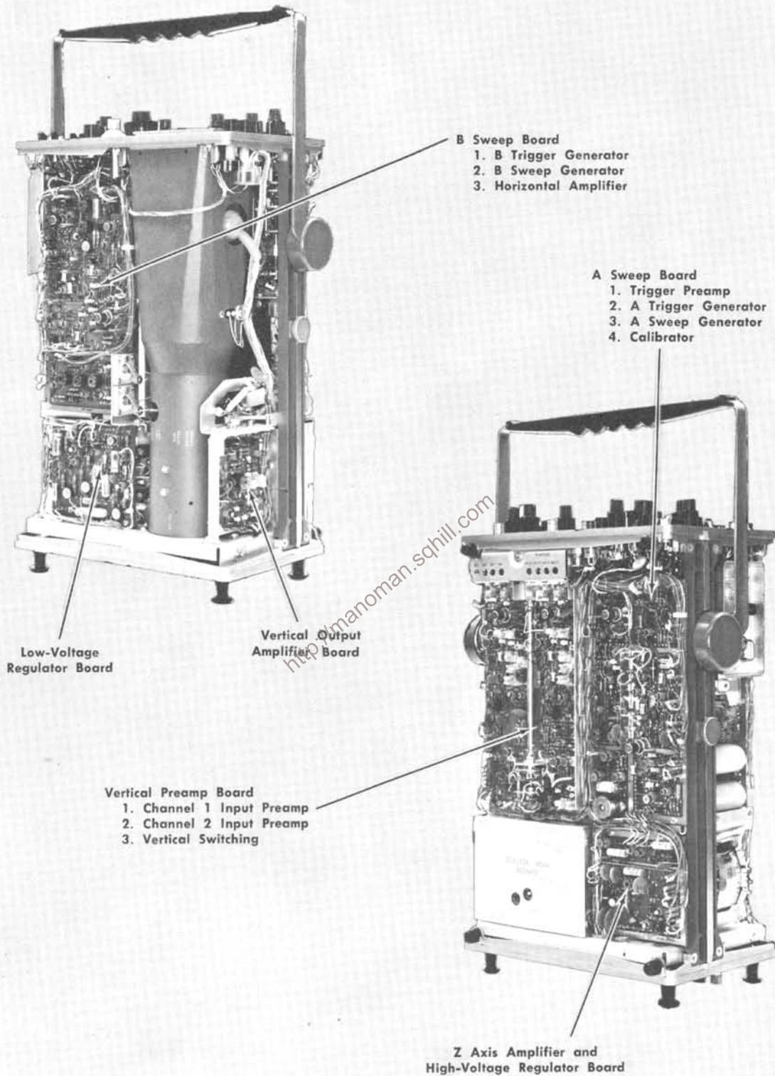
Fig. 4-4. Location of etched-wiring boards in Type 453.
