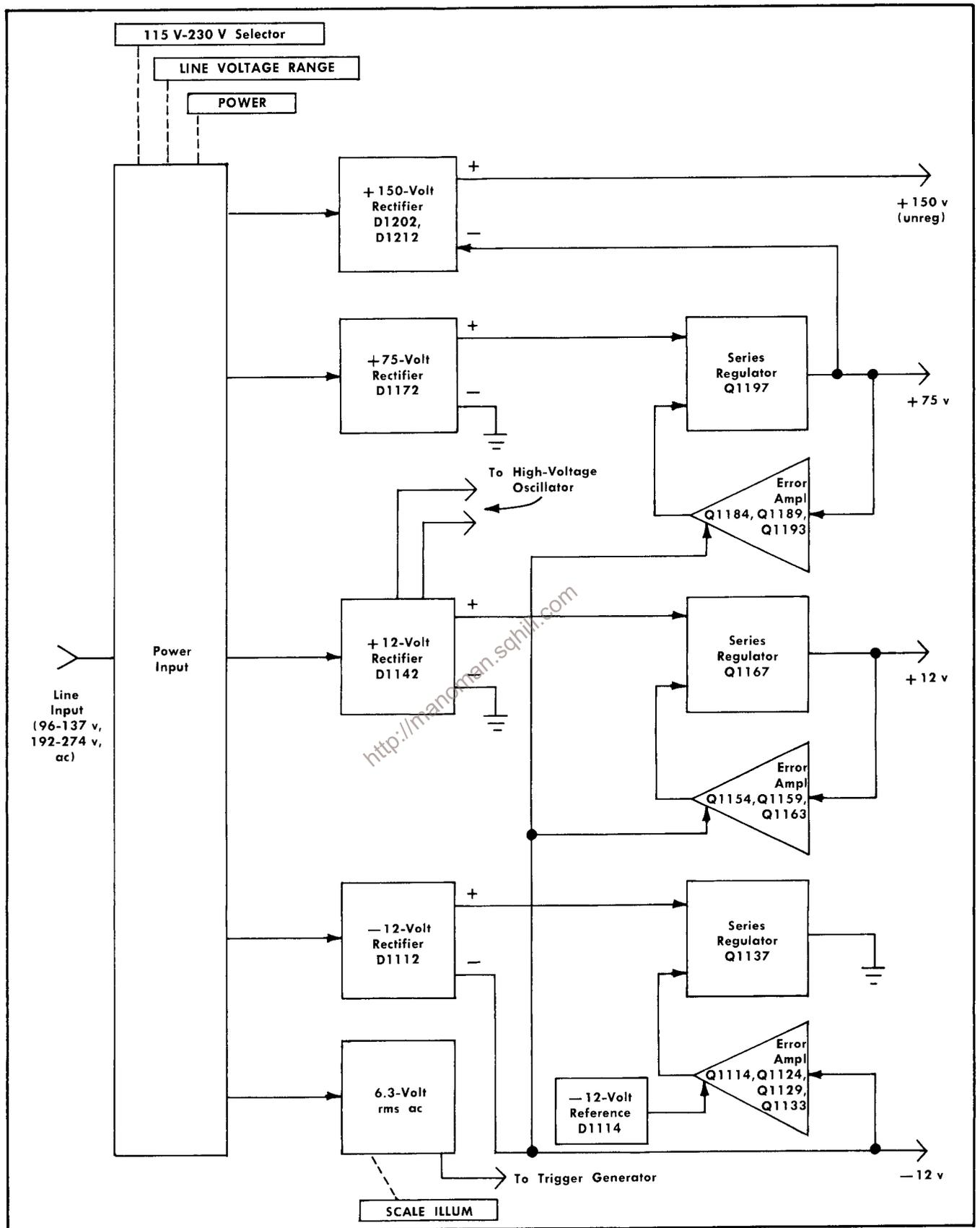
Fig. 3-13. Block diagram of Low-Voltage Power Supply circuit.
