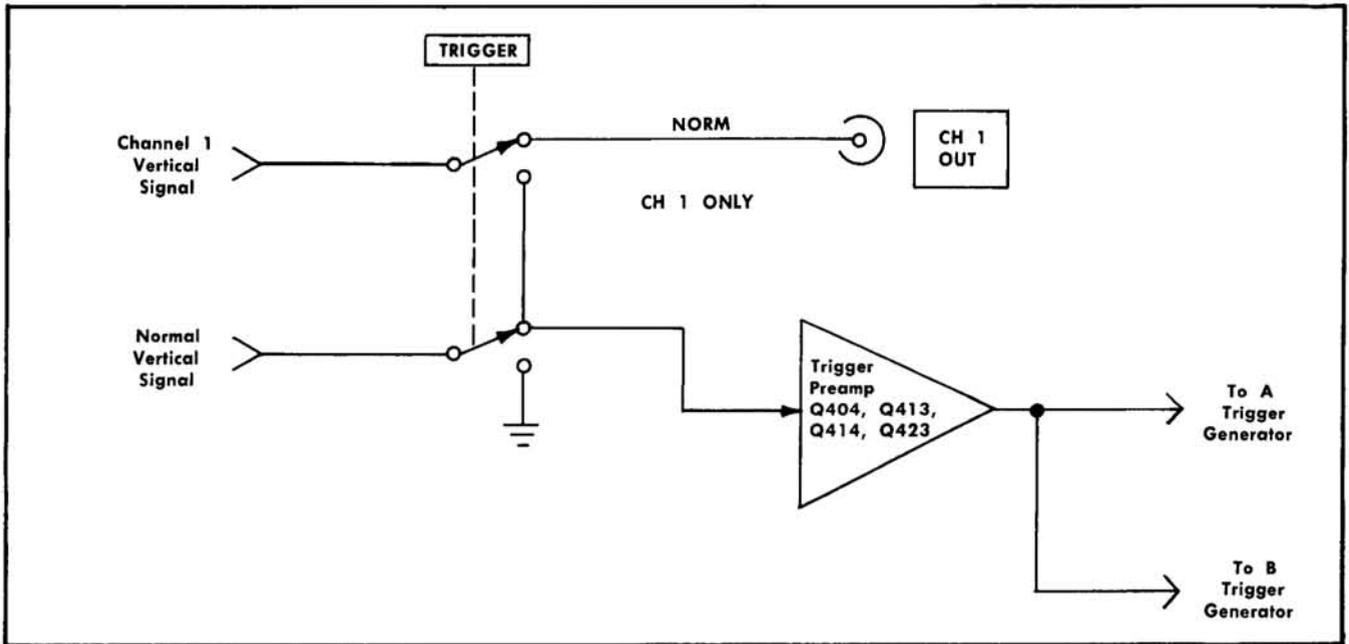
Fig. 3-5. Block diagram of Trigger Preamp circuit.
