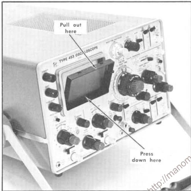
Fig. 2-5. Removing the filter or faceplate protector.
