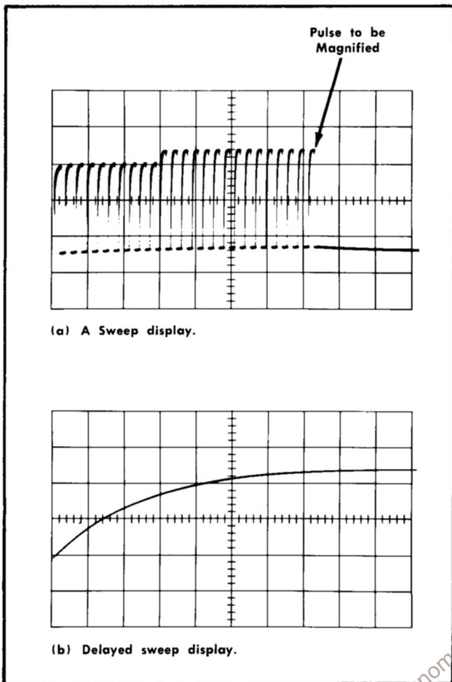
Fig. 2-20. Using delayed sweep for sweep magnification.
