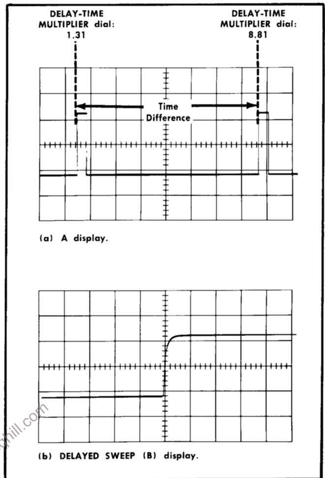
Fig. 2-19. Measuring time difference using delayed sweep.
