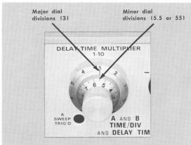
Fig. 2-12. DELAY-TIME MULTIPLIER dial. Reading shown: 3.55.
