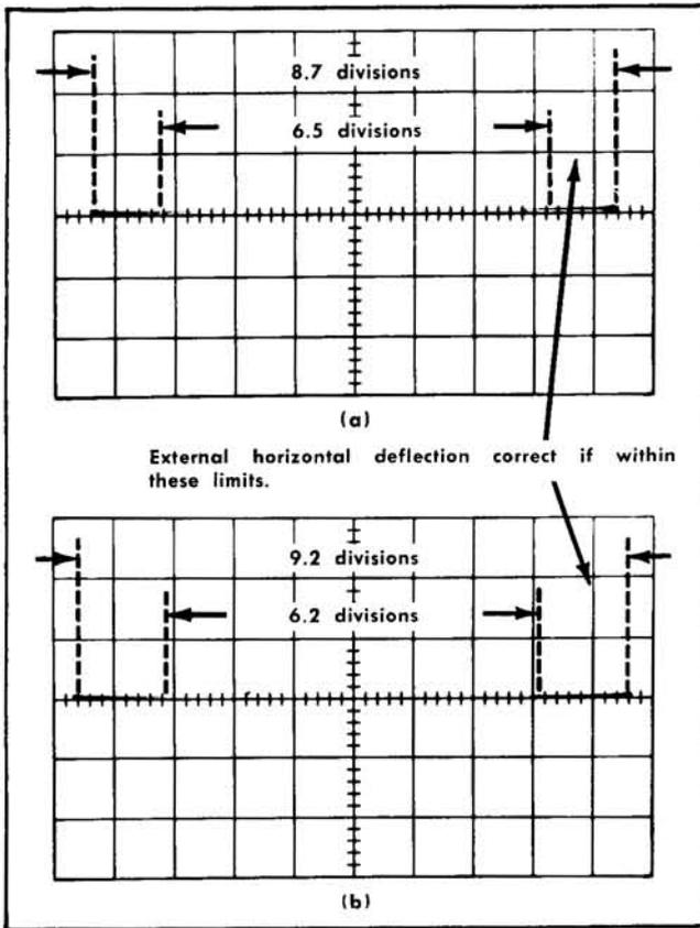
Fig. 5-20. Typical crt display when checking external horizontal deflection factor at EXT HORIZ input connector. (a) B Triggering SOURCE switch set to EXT; (b) B Triggering SOURCE switch set to EXT  $\div$  10.
