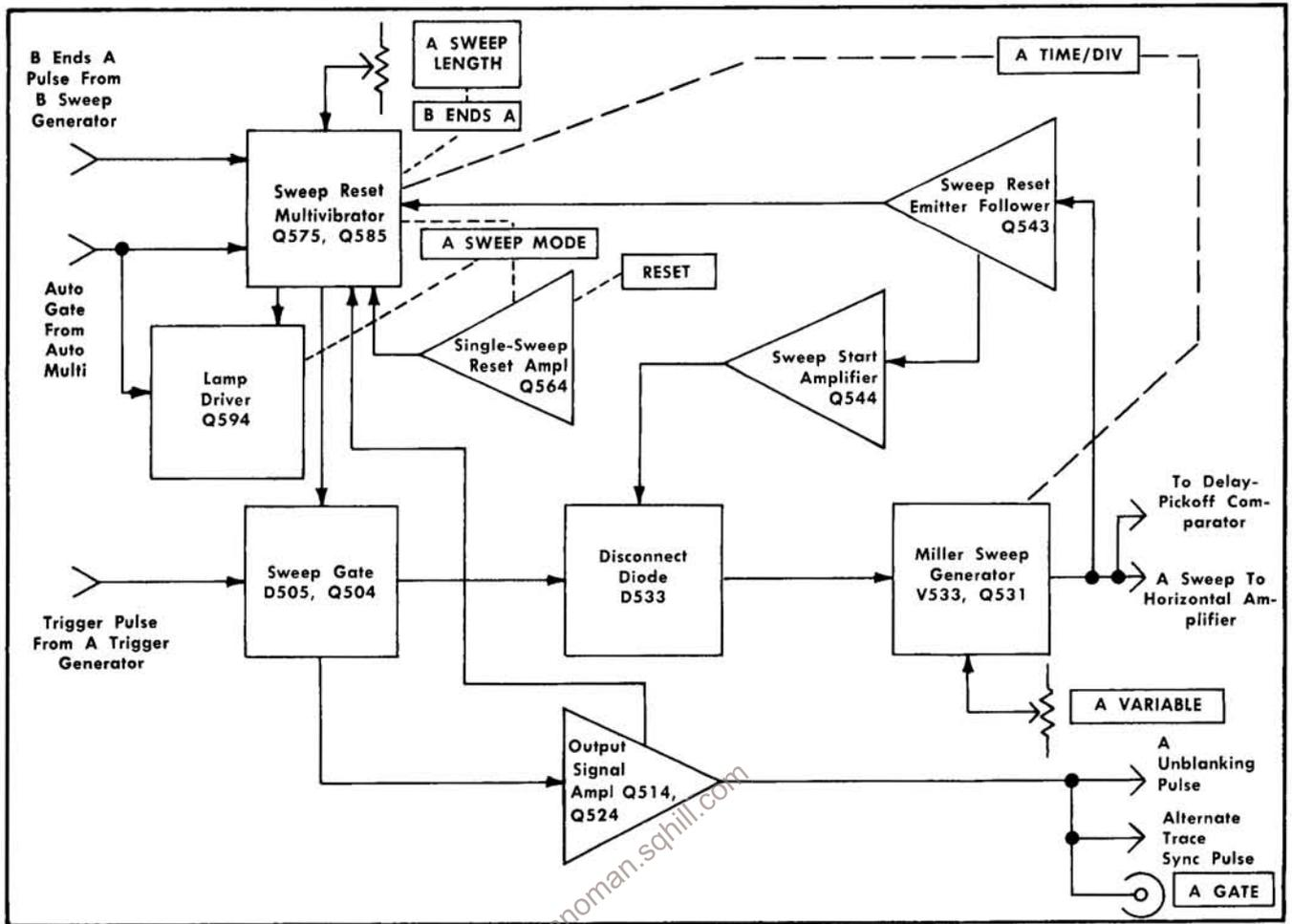
Fig. 3-8. Block diagram of A Sweep Generator circuit.
