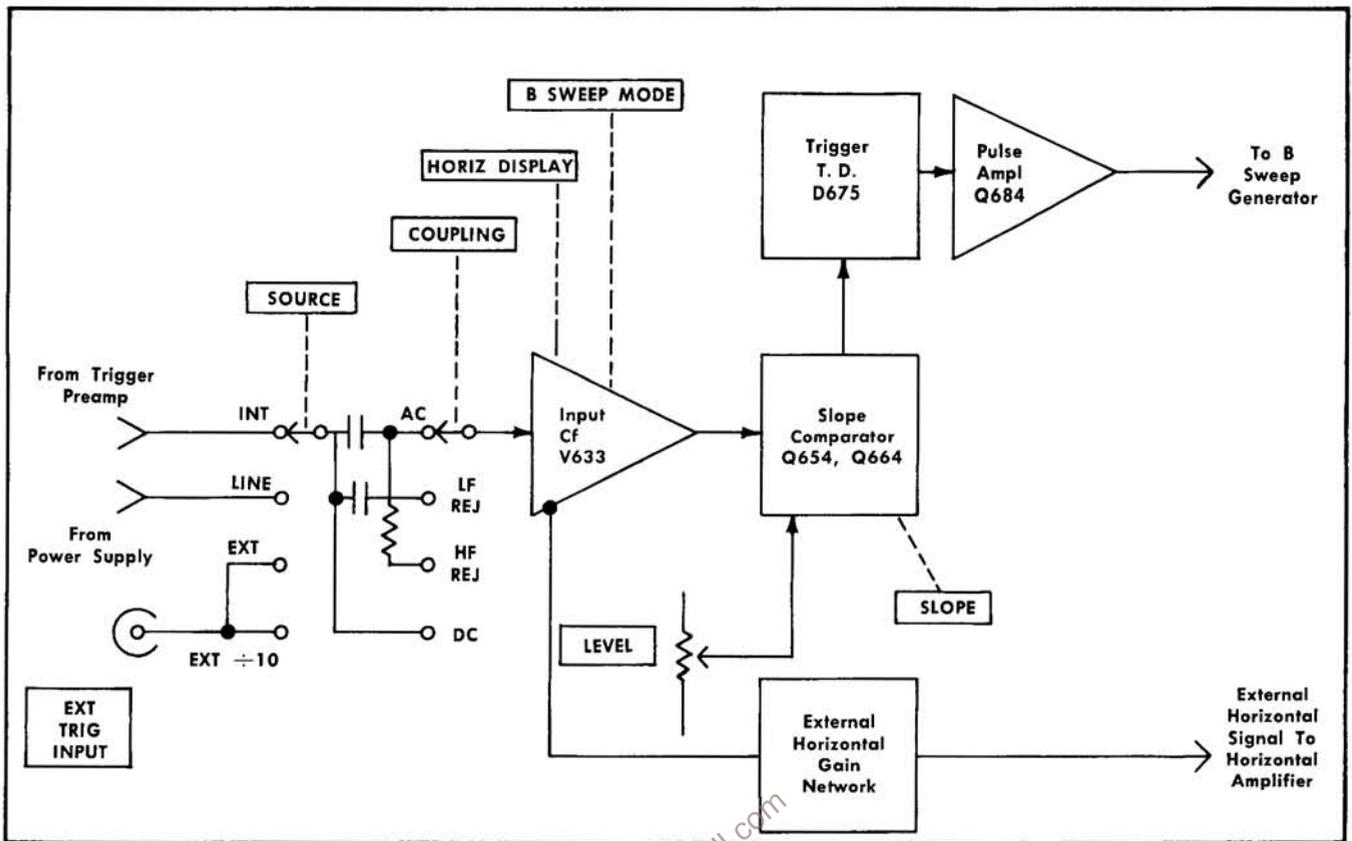
Fig. 3-7. Block diagram of B Trigger Generator circuit.
