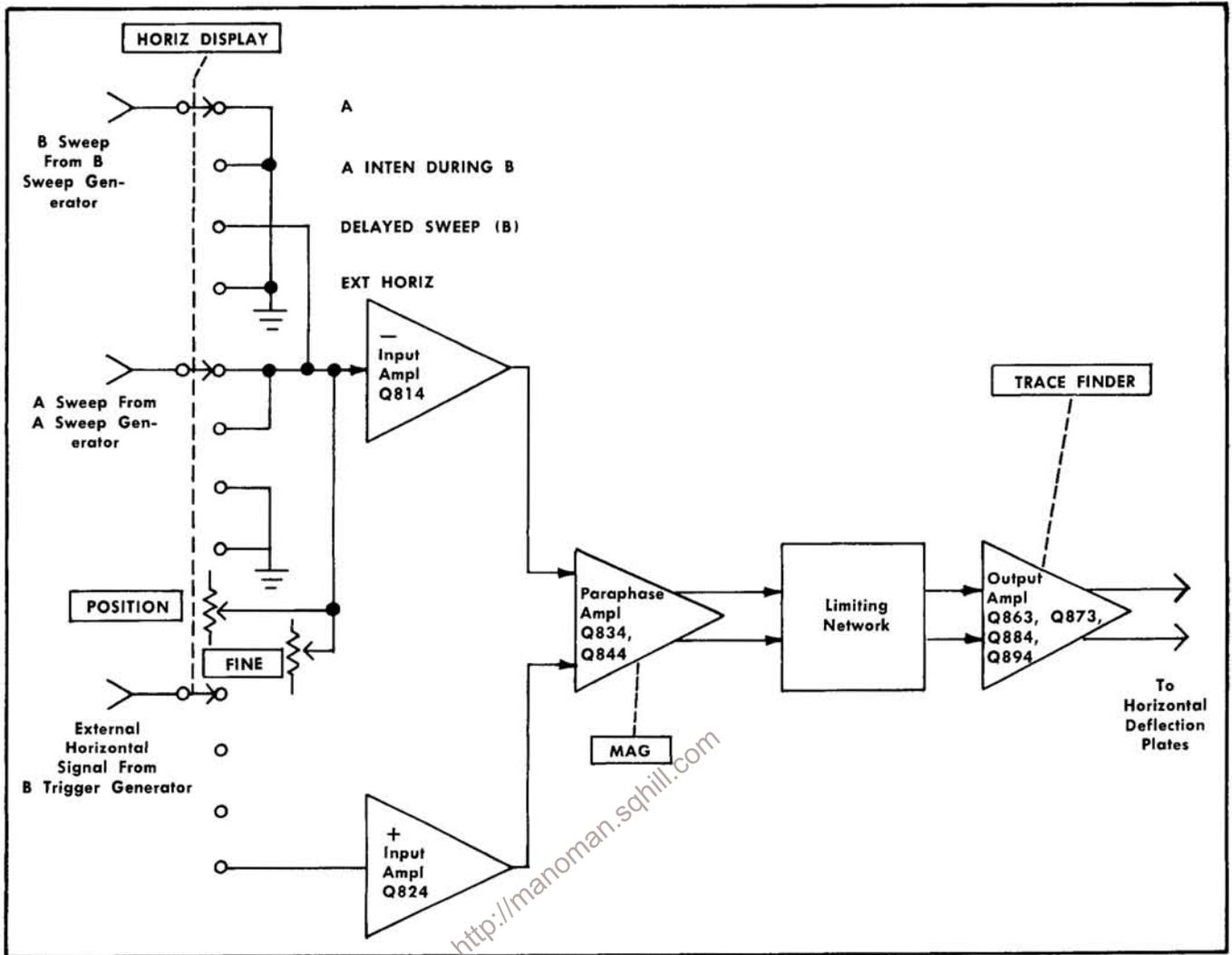
Fig. 3-10. Block diagram of Horizontal Amplifier circuit.
