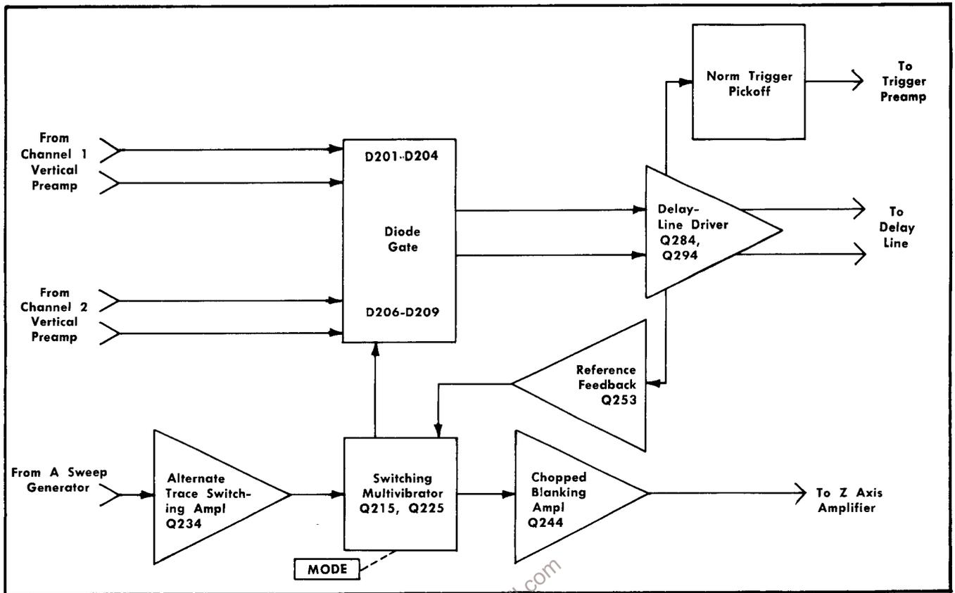
Fig. 3-2. Block diagram of Vertical Switching circuit.
