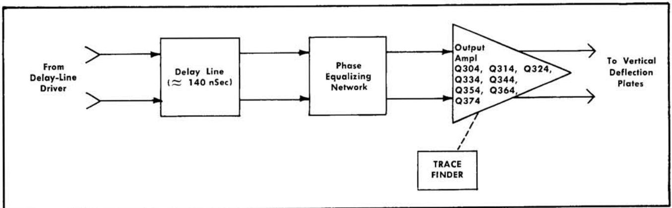
Fig. 3-4. Block diagram of Vertical Output Amplifier circuit.
